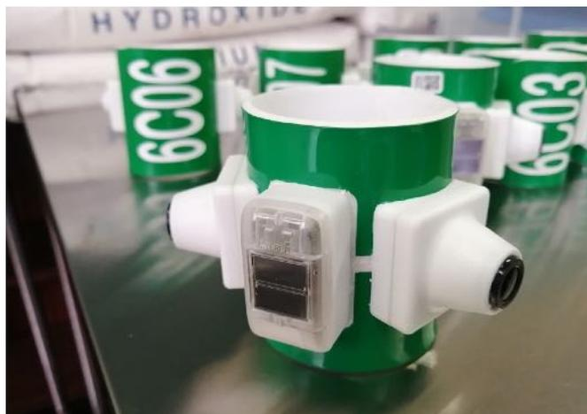
Fig. 1. GPS logger with camera (SwanEyes). The square in the center is the GPS unit, flanked by two cameras positioned at a 60-degree angle, providing a 240-degree field of view. The total weight is 130g.
